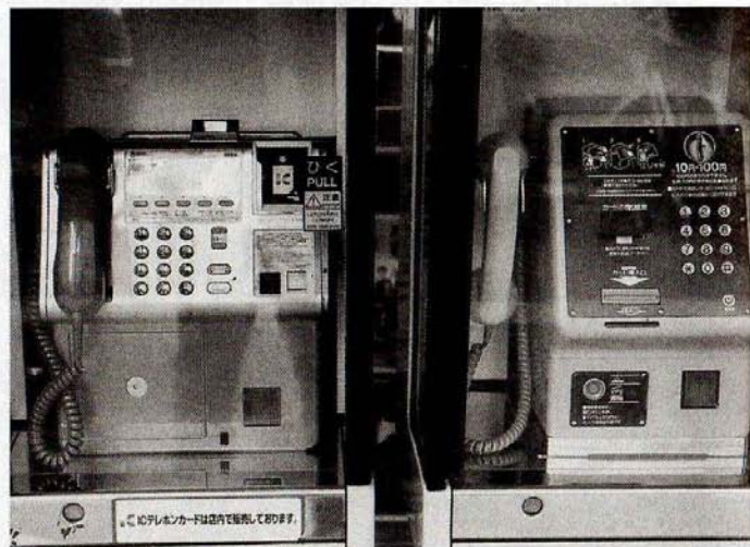
On the left is an IC card telephone for international calls; on the right a regular green, or more recently, grey, phone for domestic calls.
